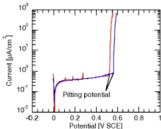
Fig. 5. Calibration scan determines pitting potential
