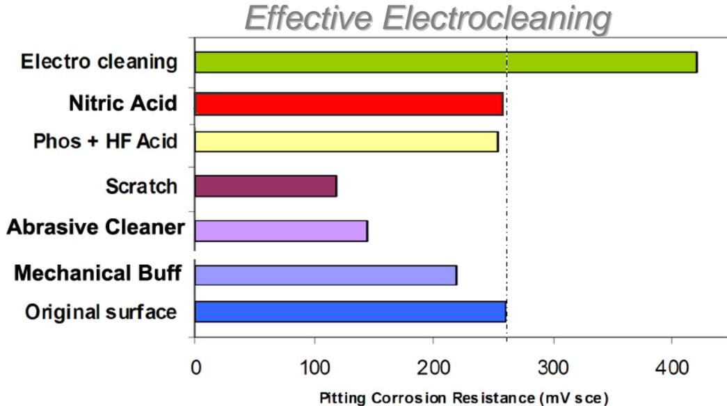
Figure 7. Comparison of the corrosion resistance of different cleaning methods.
