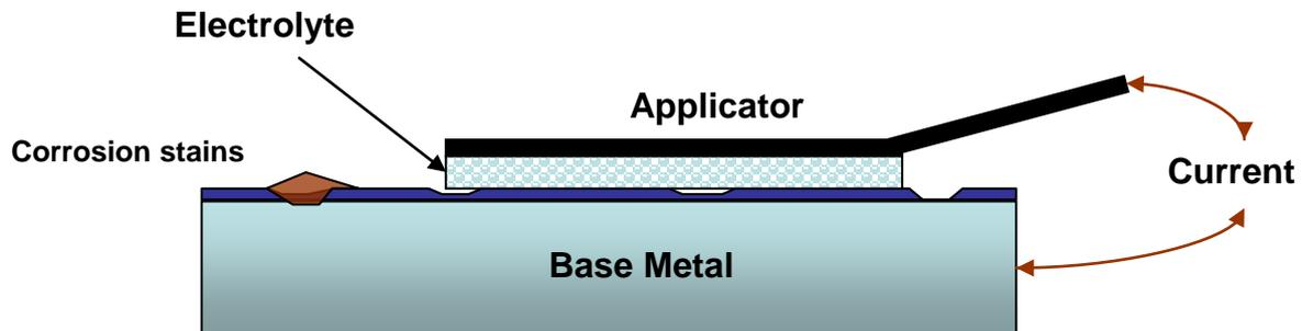
Figure 3. Electrochemical cleaning process
