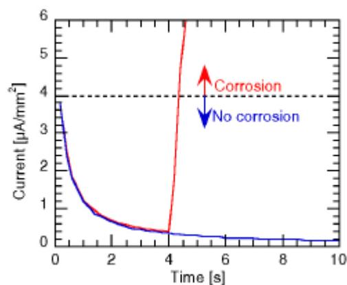
Fig.6. Corrosion current at the reference potential
